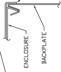
ENCLOSURE AND ACCESSORIES FASTEN TO WALL AT BOTTOM
