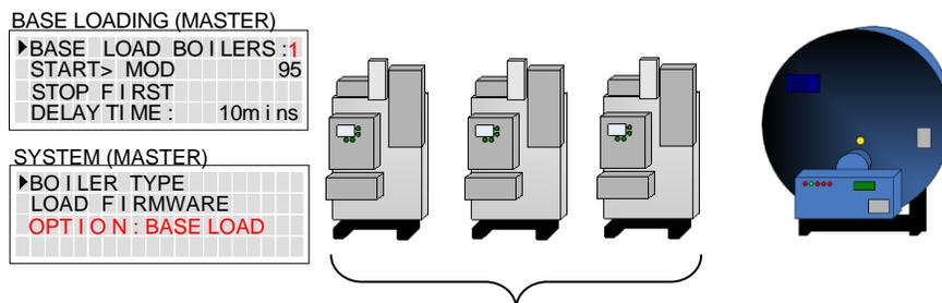
Enable the base load feature by setting:
