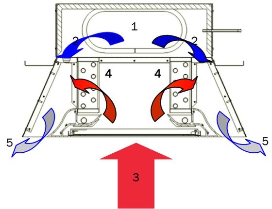
Primary air (1) is introduced into the Active Chilled Beam through a series of nozzles (2). Due to the fluid dynamic properties of nozzles, room air (3) is drawn into the Active Chilled Beam through a secondary water coil (4) by an induction process.
