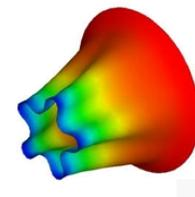
Due to the new nozzle design and increased entrainment ratios, DADANCO is able to utilize more heat transfer surface. This dramatically increases cooling and heating output of the DADANCO units for the same primary airflows.
